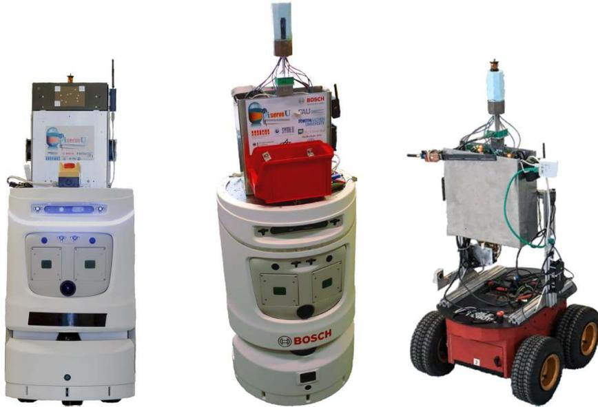
(a) Demonstrator robot platform with two radar nodes with planar arrays
